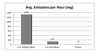
Mass Emission Testing – Average Emissions per Hour (mg) Additional full lab tests in an eight cartridge dust collector and atomite for test dust, ProTura nanofiber technology emitted 75 -98% less contaminant than the OEM filters tested. The key is the nanofiber not the substrate. Superior submicron (0.3 – 1.0 microns) particle capture leads to lower emissions of contaminant.
